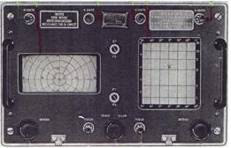
The "end" part of this equipment is the operator's indicator on which there are two screens: one showing relative height of the target and the other showing relative bearing.
